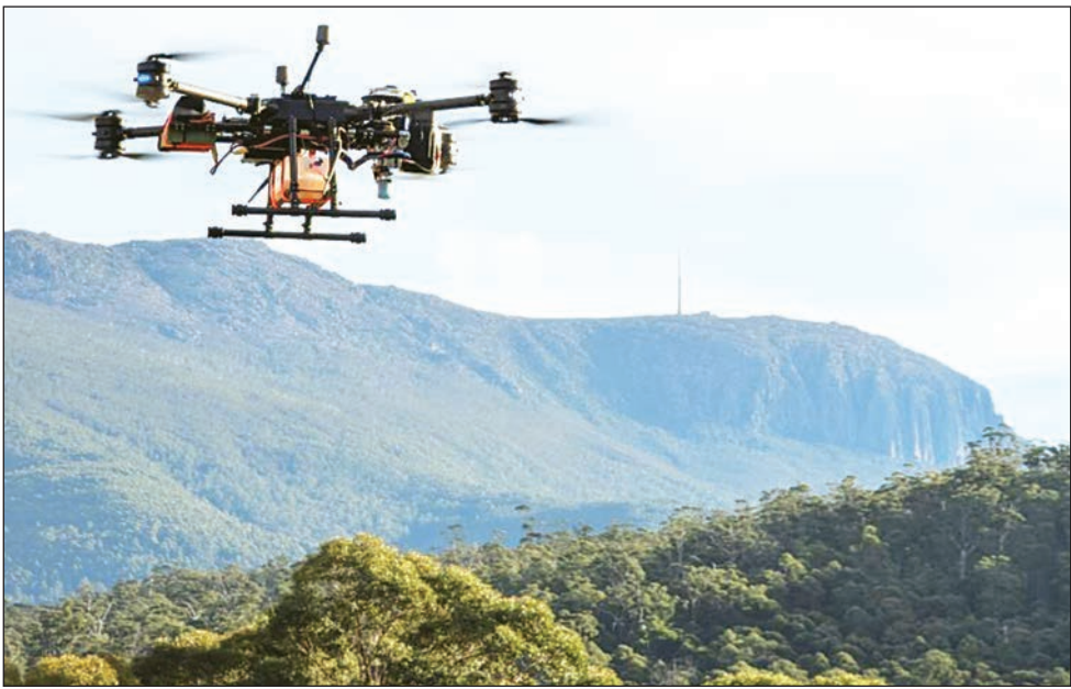
Huntingfield-based Currawong Engineering is excited to share their new 'hybrid engine' technology at the convention. This engine charges Unmanned Aerial Vehicle batteries during flight. (PS)
